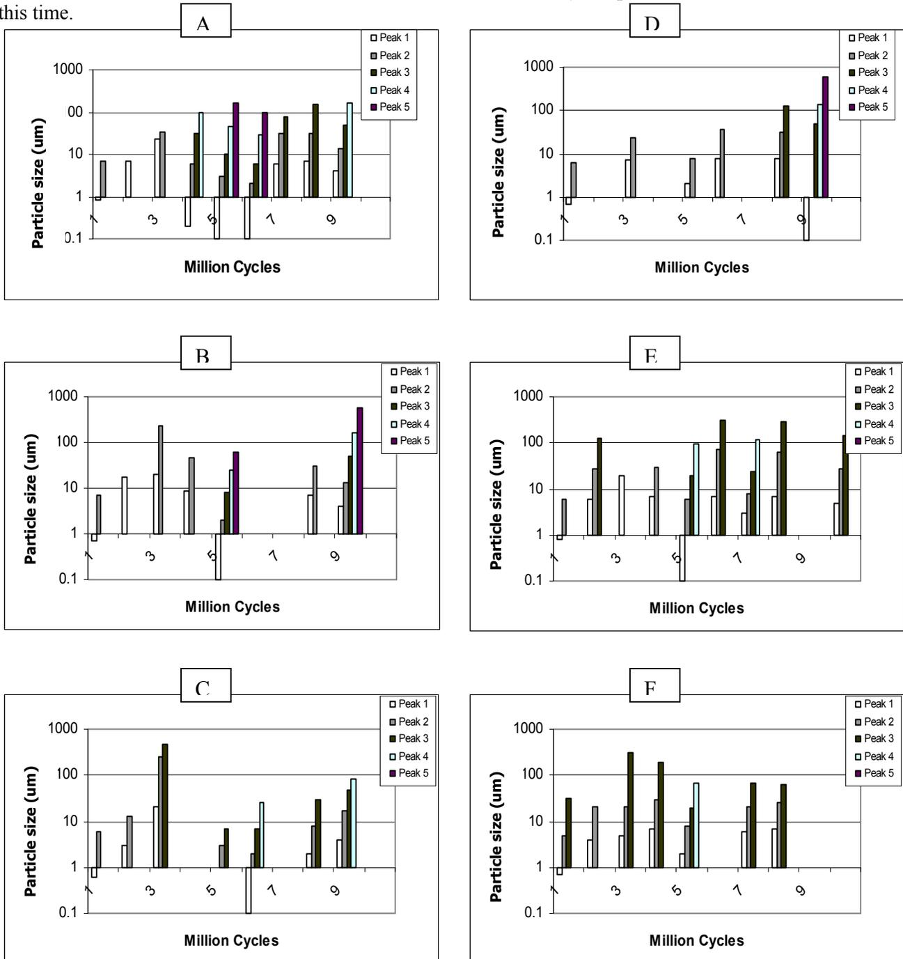
Figure 1. Graphical representation of the number of peaks within each particle size distribution and their associated particle size for each of the six specimens over the course of testing. Variation in the number of peaks over the course of testing shows the heterogeneity and complexity of wear debris production was consistent and that a reduction in wear to a single peak (particle size) did not occur in any of the specimens.
