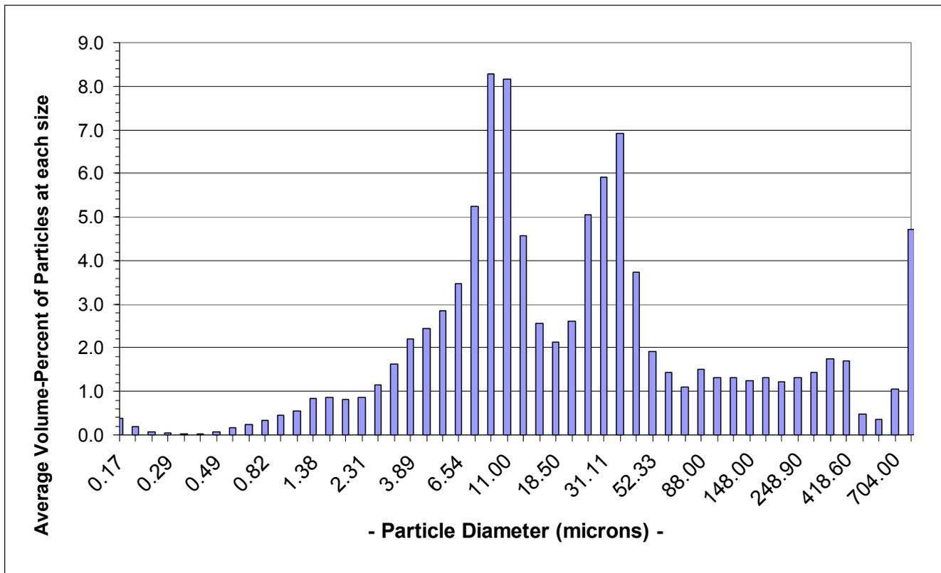
Figure A. The average volume-based percent distribution of particle sizes for 6 samples over 10 million cycles.
