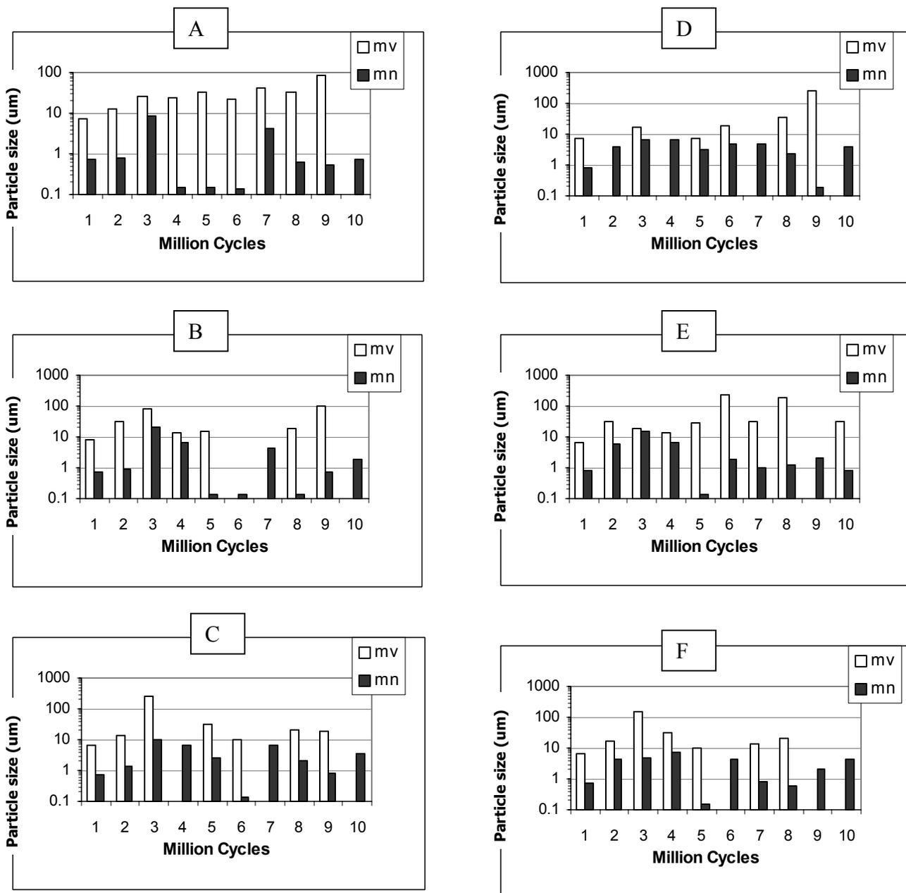
Figure 2. Graphical representation of the average particle size using both mv (volume) and mn (number) analysis, for each of the six specimens over the course of testing.
