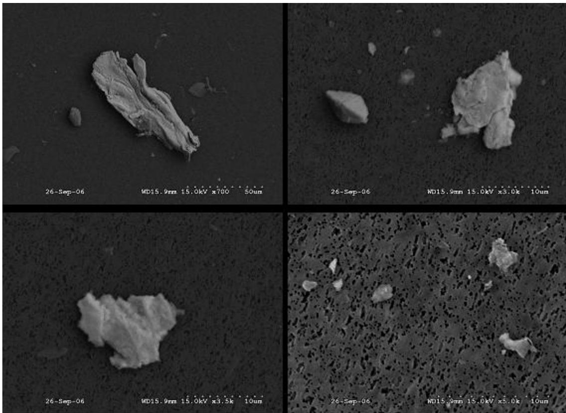
**Figure E.** Examples of metal particles from sample D (4 million cycles) showing flake and granular particle morphology.
