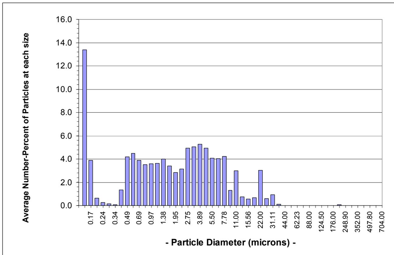
Figure B. The average number-based percent distribution of particle sizes for 6 samples over 10 million cycles.
