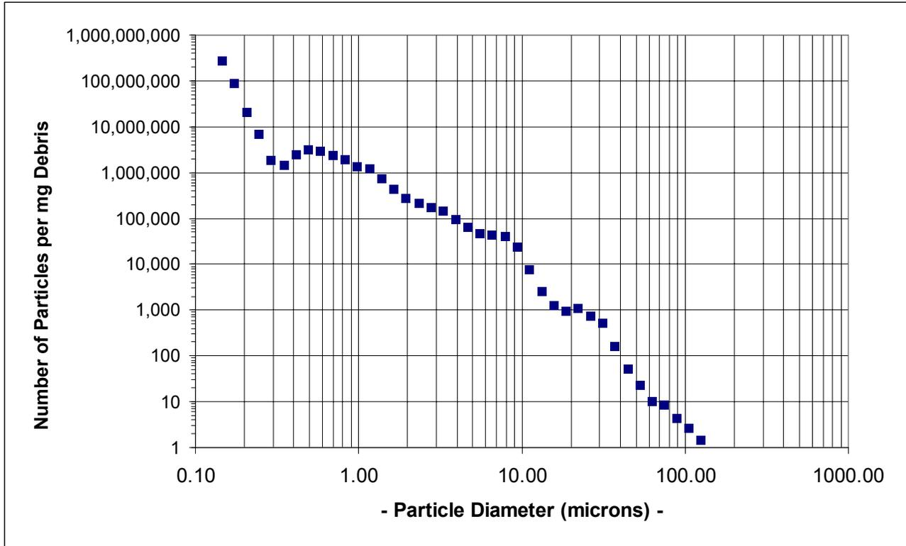
**Figure C.** A distribution showing an average of the total number of particles for each particle size per mg of wear.
