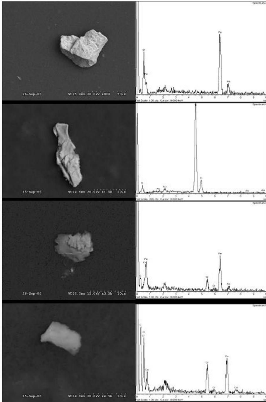
**Figure F.** Examples of typical particles EDAX identified as Fe-oxide, Ti-alloy, steel and Co-alloy (Top to Bottom) from sample simulator fluids (Note Au and PD were used for sputter coating specimens for SEM). Generally the Co-alloy particles tended to be smaller and more granular in shape (<10um), but were not heavily oxidized, i.e. not likely corrosion products.
